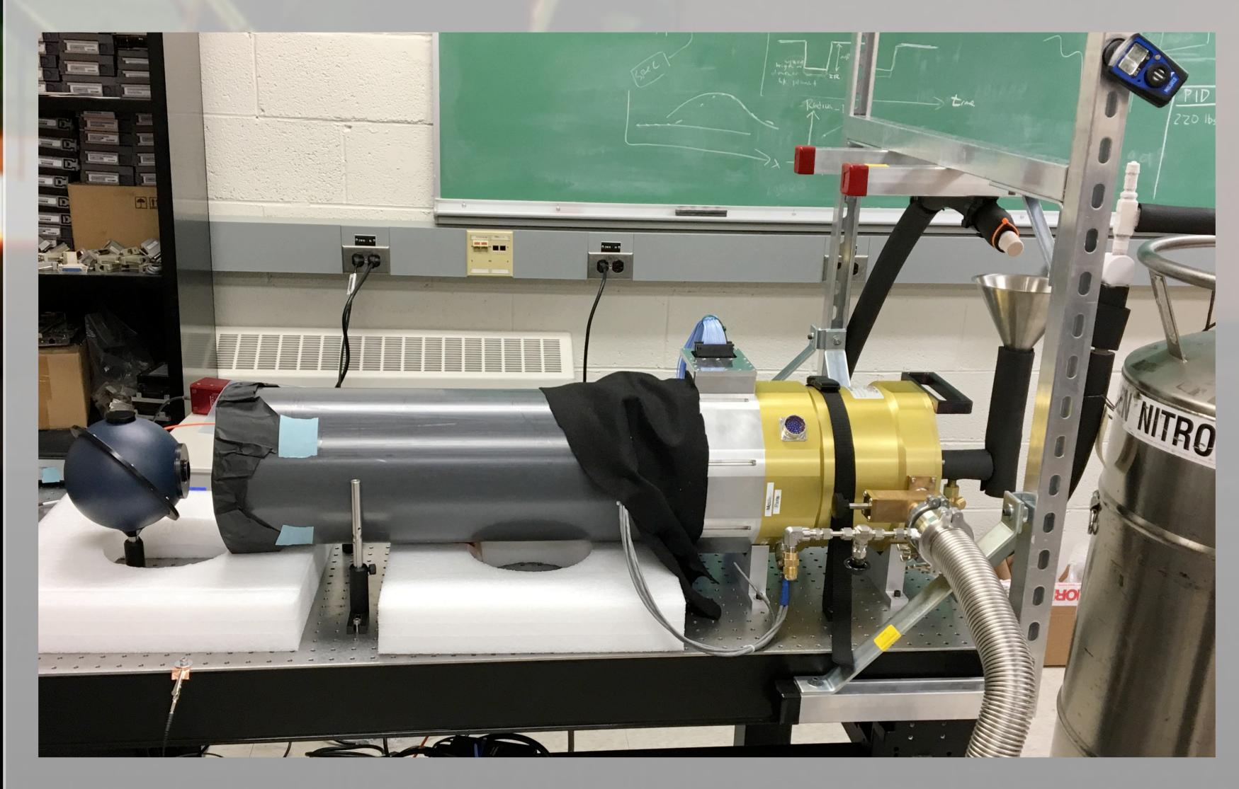
The CCD characterization lab. The CCD is cooled to -100 °C in an LN2 Dewar with an auto-fill system. A wide range of light sources can be projected from approximately 1 m away.
