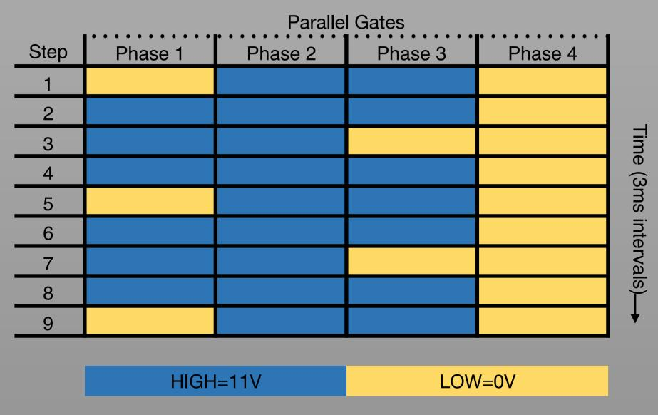
The "dither" clocking scheme takes advantage of the four CCD phases to exercise the parallel clocks during integration without moving charge between pixels.
