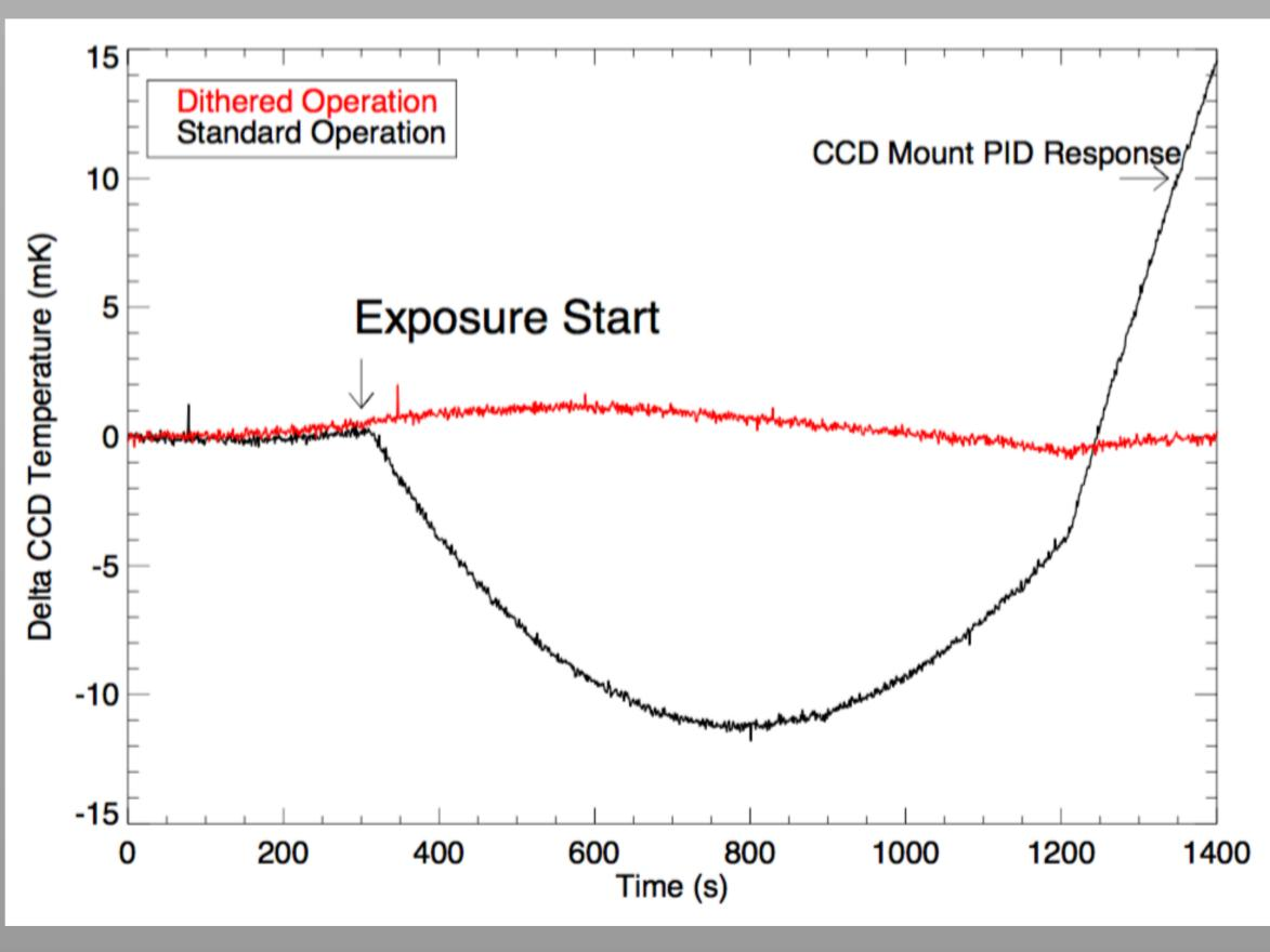
variations of the CCD package during integration and readout are significantly smaller using the "dither" clocking scheme. Prelim-
