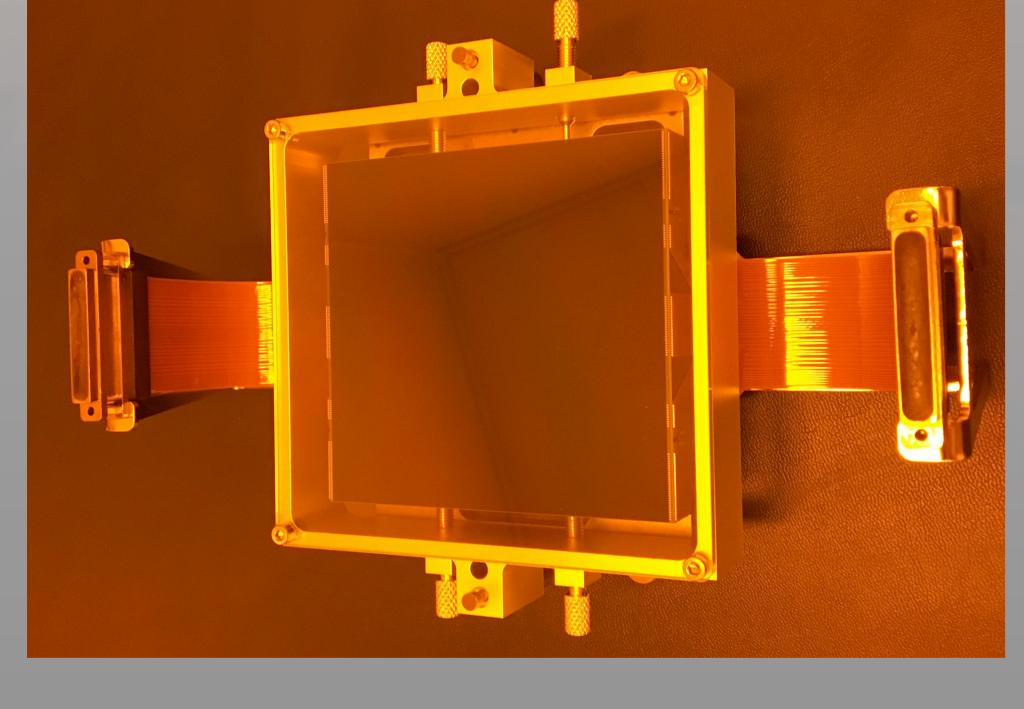
A CCD290-99 in our custom handling jig. The CCDs are installed into our test Dewar within a Class 100 Cleanroom. The CCD is ~90 mm<sup>2</sup>.
