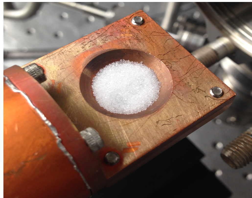
Lab sodium chloride after irradiation with electrons.
