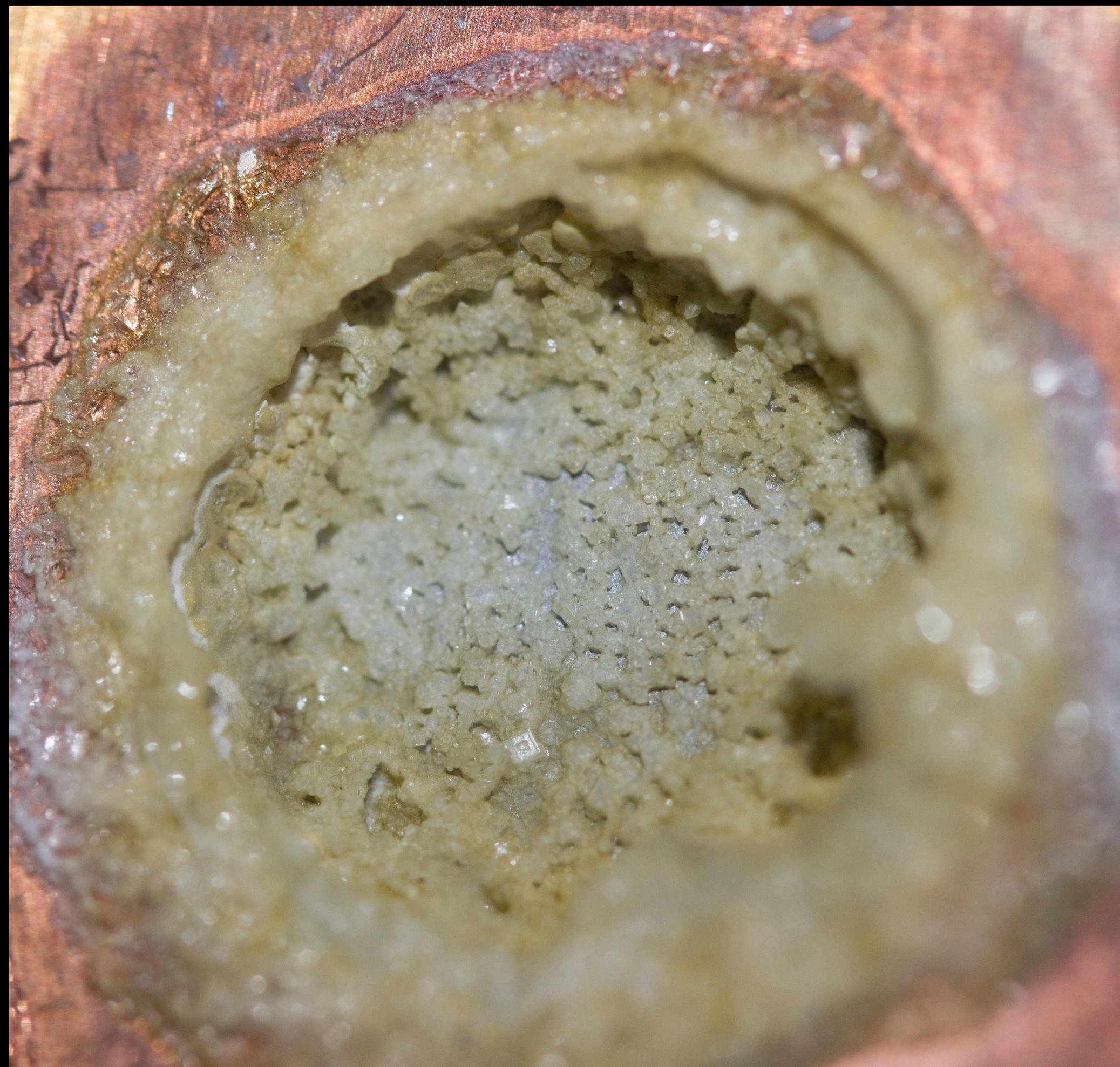
Sodium chloride brine evaporite post-irradiation
