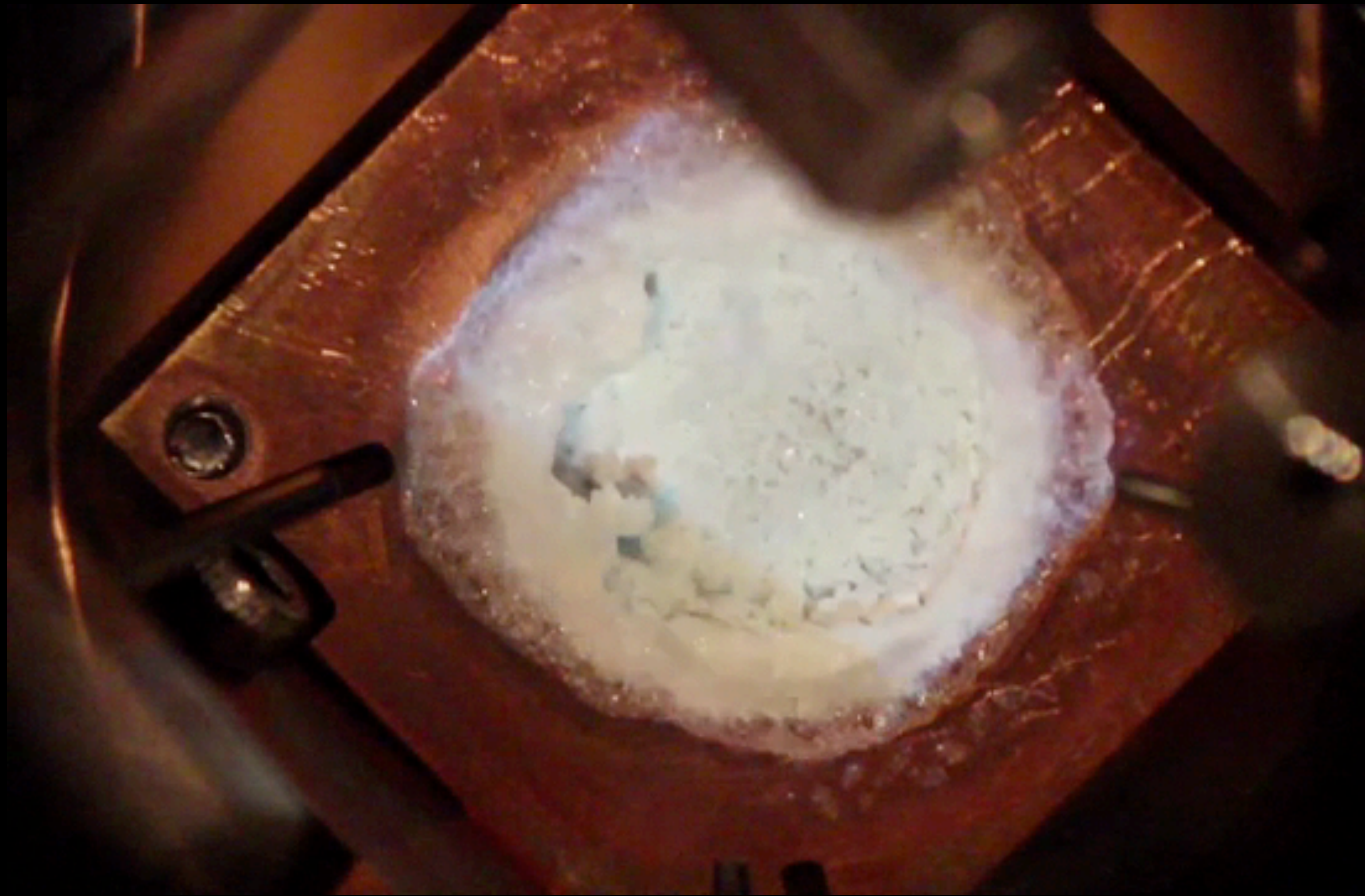
NaCl evaporite. T = 100 \text{ K} , P = 1\text{e-}9 \text{ Torr} , 10 \text{ keV} electrons
