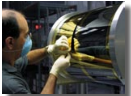
A prototype mirror segment for Constellation-X being separated from the replicating mandrel.
